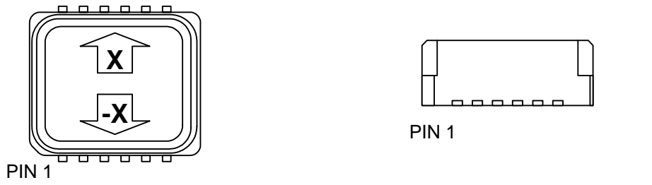
Figure 2. Accelerometer measuring directions
